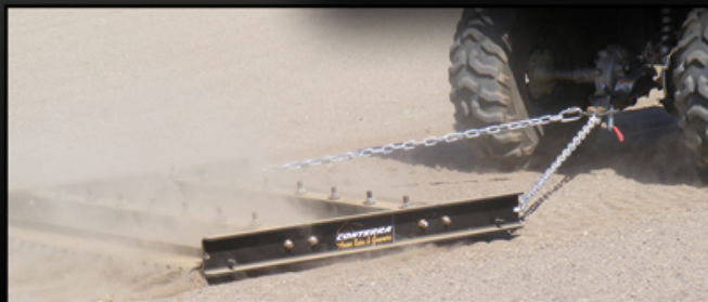
Swept tines help the Drag maintain contact with the ground, reducing the bounce.
