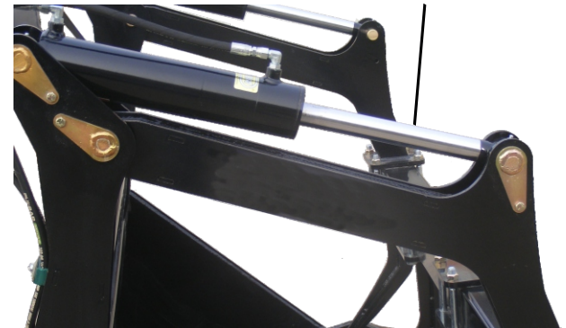
Heavy Duty 3" Ram with a 12" Stroke
