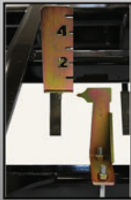
Scarifier Shank and durable, easily replaced Scarifier Teeth
