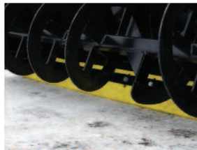
Optional urethane skid shoes (left) and cutting edge (right)
