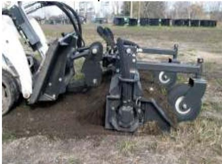
of faster ground speed. The counter rotating rotor moves soil ahead of it as it tills, filling in low spots and chewing off high spots. It creates perfect seed beds and windrows. This attachment separates rocks, tears up sod and pulverizes dirt clods. It rakes and tills as deep as 2"
