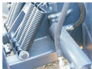
Spring Trip helps prevent blade damage
