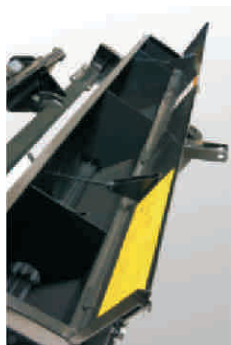
The seed box utilizes a newly designed blade type agitator.
