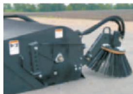
Optional Curb Sweeper Can be moved up when not in use
