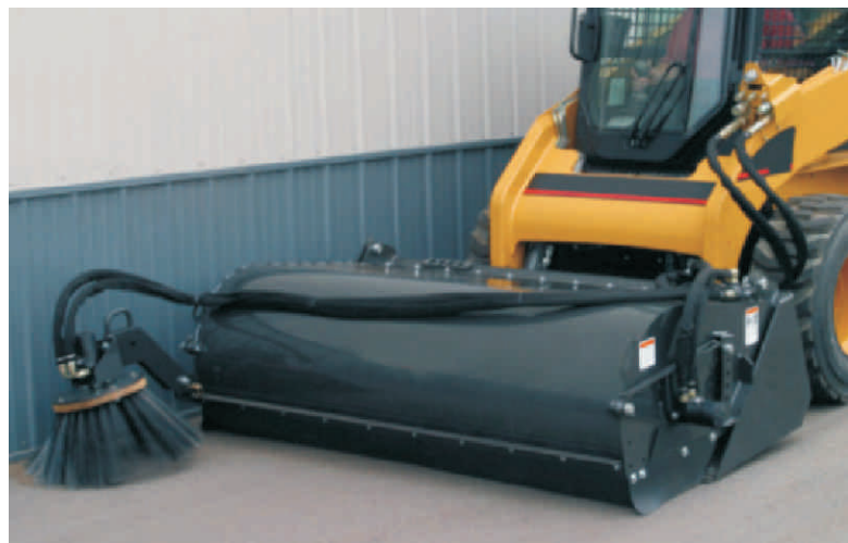
Shown with optional curb sweeper for getting closer to curbs, buildings or other objects.
