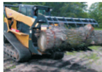
Gusseted between teeth for added strength.
