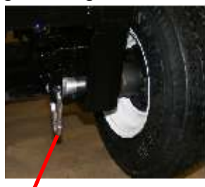
Locate Depth Wheel Adjustment retainer Pin
