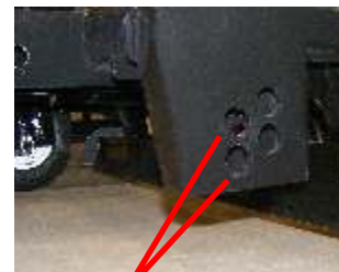
Select new wheel depth and re affix wheel at new depth
